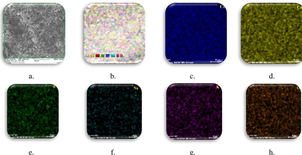
**Figure 3.** Distribution of Co, Cr, W, Mo, Na, K and O elements: a) surface under analysis, b) distribution of all elements on surface, c) Co, d) Cr, e) W, f) Mo, g) Na, h) K, i) O
