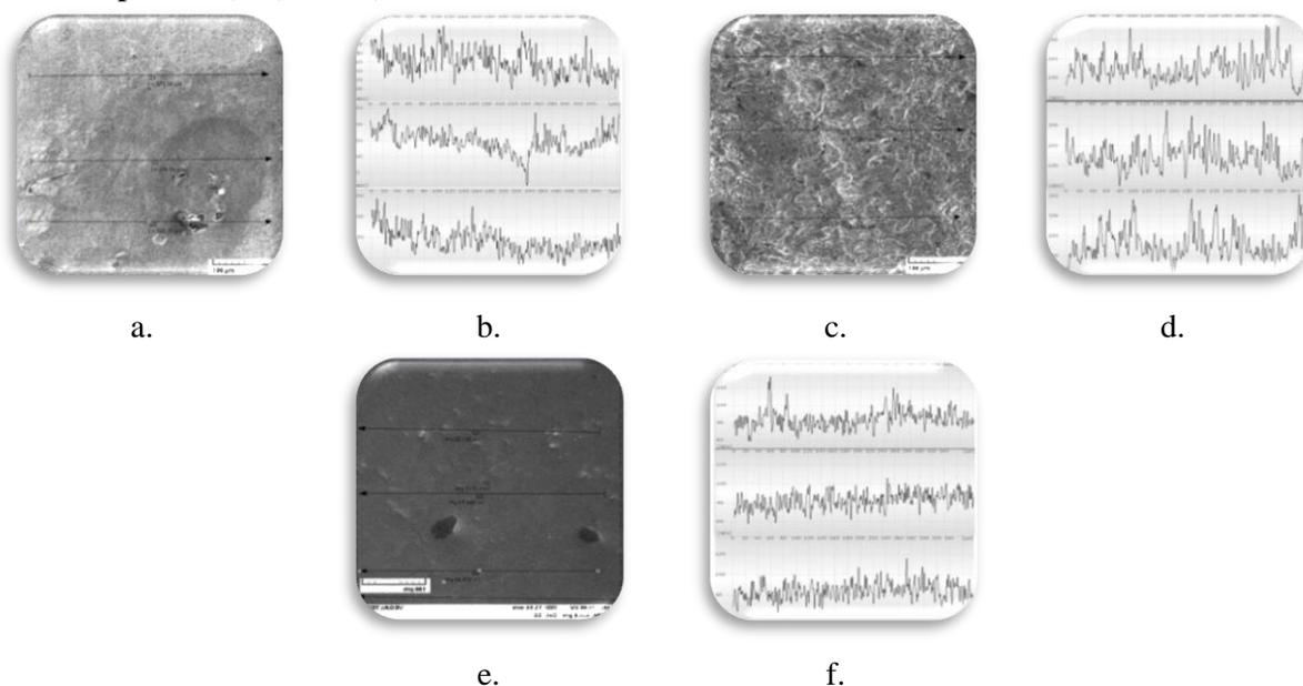
**Figure 1.** SEM images of the surfaces of experimental specimens after the electrochemical corrosion test: a) NS specimen at 500:1 power b) rugosity of NS specimen, c) 1S specimen at 500:1 power, d) rugosity of 1S specimen surface, e) 2S specimen at 500:1 power, f) rugosity of 2S specimen surface
